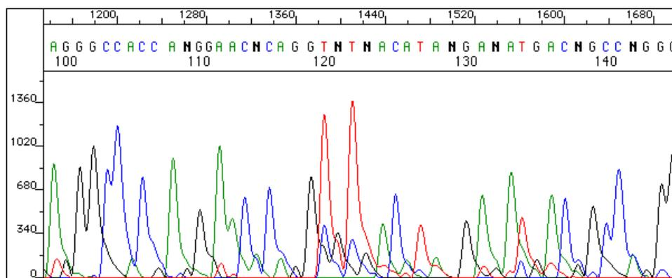
**Figure 7-59** Trailing peaks caused by capillary failure
