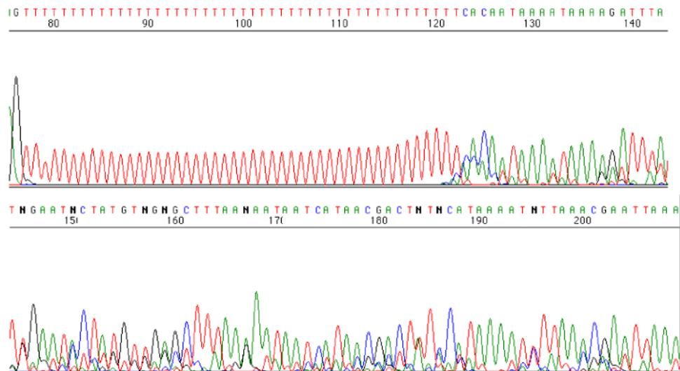
**Figure 7-45** Homopolymer region sequenced using BigDye terminator chemistry
