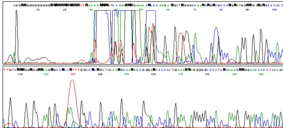
**Figure 7-68** Incorrect Peak 1 Location and Start Point (both set to 963 scans)
