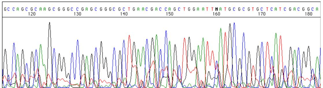
**Figure 7-65** BigDye terminator data collected with a Filter Set E run module and analyzed with an incorrect (Filter Set A) instrument file
