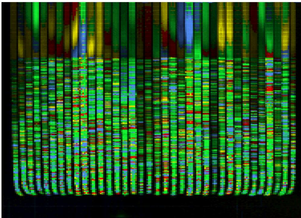
**Figure 7-54** Electrophoresis failure caused by a buffer leak
