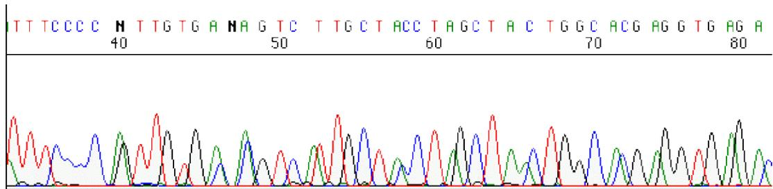
**Figure 7-14** BigDye terminator data analyzed with a BigDye primer dye set/primer (mobility) file, which results in poor mobility correction
