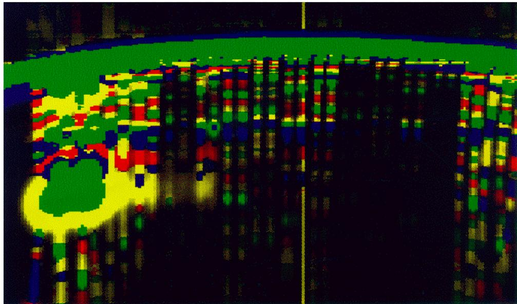
**Figure 7-52** Fluorescent contamination from a marking pen
