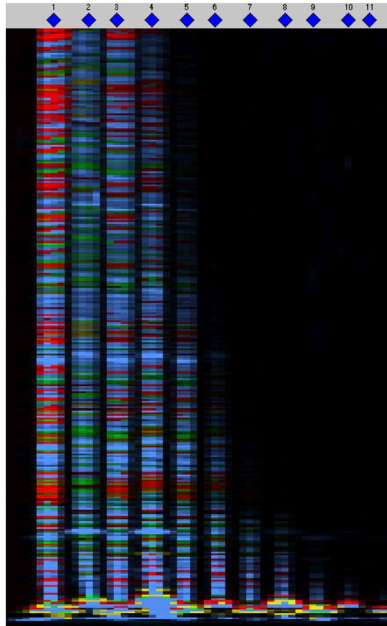
**Figure 7-32** Effect of contaminating NaCl on sequencing data
