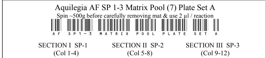
All plates are labeled with ToughTags in both text and machine readable bar code fonts. The label is affixed to the front of the plate.
